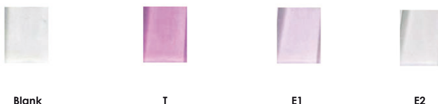
Figure 2: demonstration of the competitive effect of N-hydroxysuccinimide vs. ferrospectral on iron.
